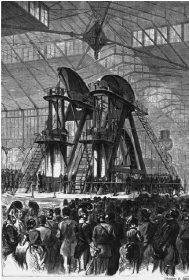
The American System of political-economy created the greatest industrial power the world had ever seen. Here, a Corliss engine at the 1876 U.S. Centennial Exhibition.
